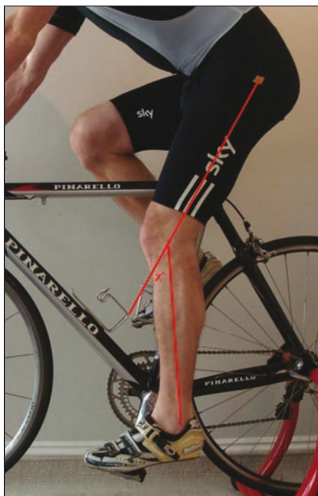
Figure 2. Determining the knee angle ( x degrees) at the bottom of the pedal stroke using the "Holmes method".
